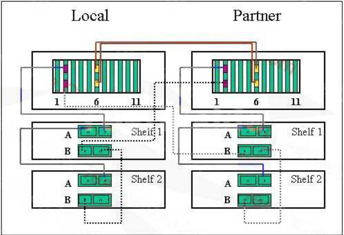
Is this standard clustered pair properly cabled based on Network Appliance's standard cabling recommendation for the FAS900 series?
