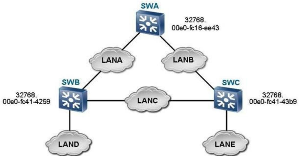
As shown in the figure, when the STP network runs properly, which device does the designated port of LANC reside?
