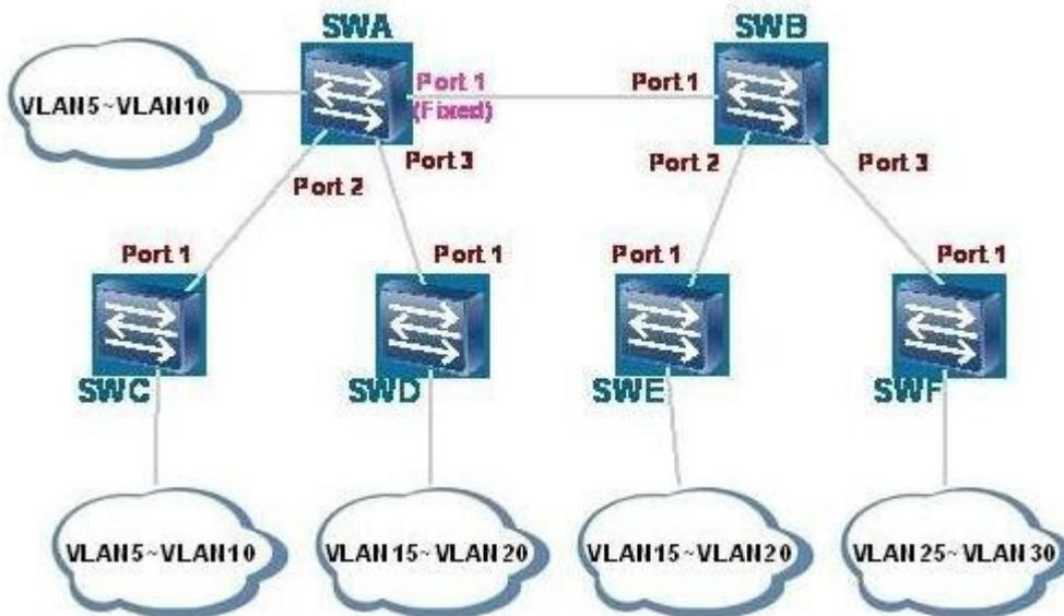
As shown in the figure, port 1 of switch A is configured with the Fixed mode, and other ports are configured with the Normal mode. The trunk interfaces allow all VLANs. Which VLANs are registered on port 1 of switch C? (Select 3 Answers)
