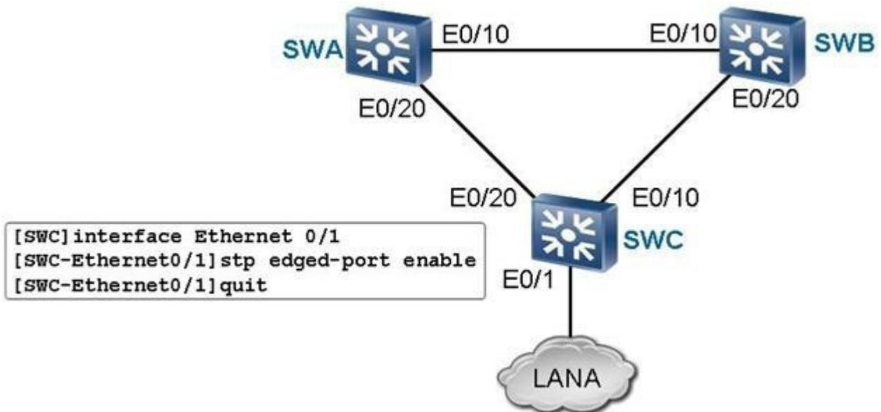
On the RSTP network as shown in the figure, what is the port role of SWC E0/1 according to the configuration? (Select 2 Answers)
