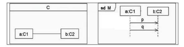
A. The communication diagram on the left forms the base for the sequence diagram on the right.
