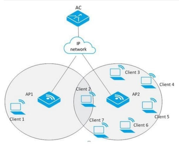
The access controller (AC) has configured session-mode load balancing. The maximum number of sessions is configured as 5. The maximum session gap is configured as 4. Client 1 is associated with API Clients 2 to 6 are associated with AP2. Client 7 can only hear AP2. Client 7 attempts to associate to AP2.
