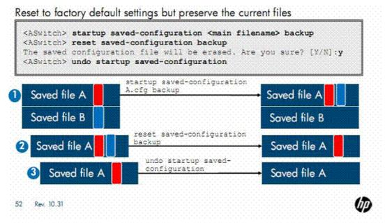
Sometimes you will need to revert a switch to its factory-default settings, but the customer still wants to preserve the current startup-config file (or files). You can meet this requirement with one command when the switch has no backup startup-config. Simply enter the undo saved configuration command, which removes the main attribute from the main startup-config file, but preserves the file itself. When the switch reboots, it loads the
