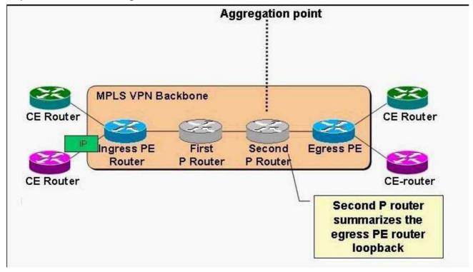
A.The first P router will be faced with a VPN label which it does not understand.
